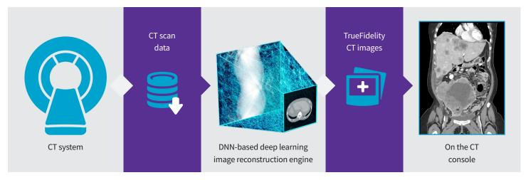
Figure 8: Reconstruction flow of deep learning image reconstruction.
