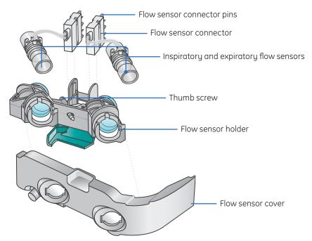
Figure 11.4 Flow Sensor Components
