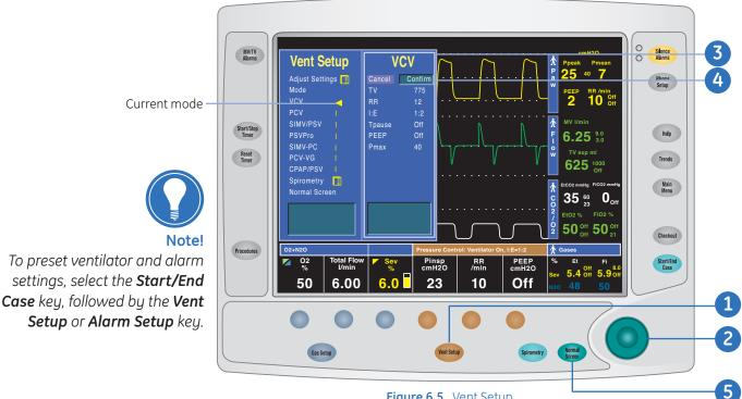
Figure 6.5 Vent Setup
