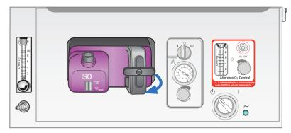
Figure 4.5 Remove the Aladin<sub>2</sub> Cassette
