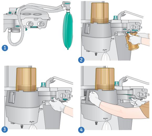
Figure 11.1 Removing the Breathing System
