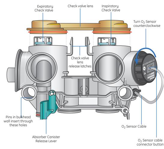
Figure 11.6 Removing the Breathing Circuit Module
