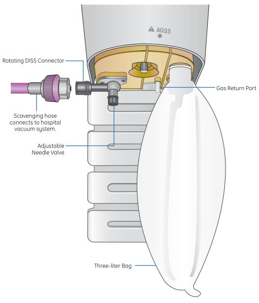
Figure 2.14 Active Adjustable Flow
