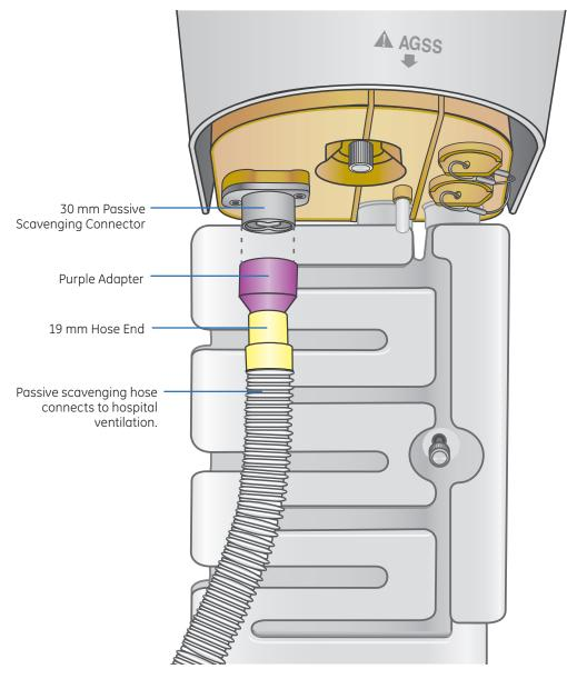
Figure 2.12 Passive Anesthetic Gas Scavenging System
