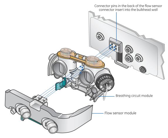
Figure 11.5 Replacing the Flow Sensors
