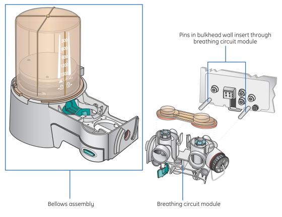
Figure 11.7 Replacing the Breathing Circuit
