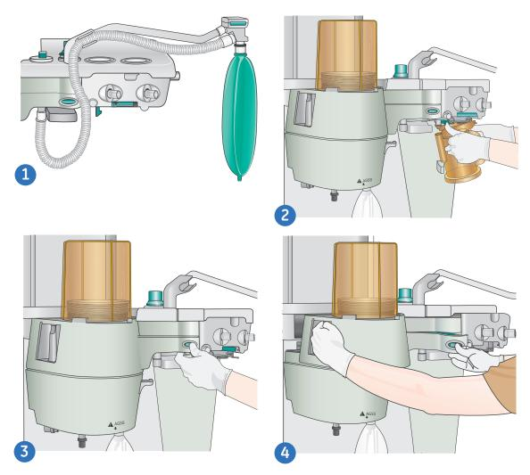
Figure 11.1 Removing the Breathing System
