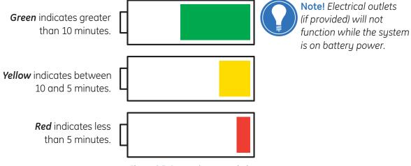
Figure 2.7 Battery in use symbol
