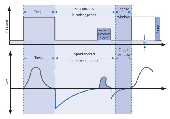
Figure 7.5 Example of SIMV-PCV Waveforms
