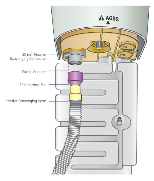
Figure 2.15 Passive Anesthetic Gas Scavenging System
