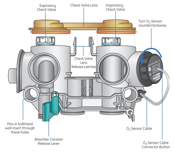
Figure 11.6 Removing the Breathing Circuit Module
