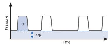
Figure 7.8 Example of CPAP + PSV Waveforms
