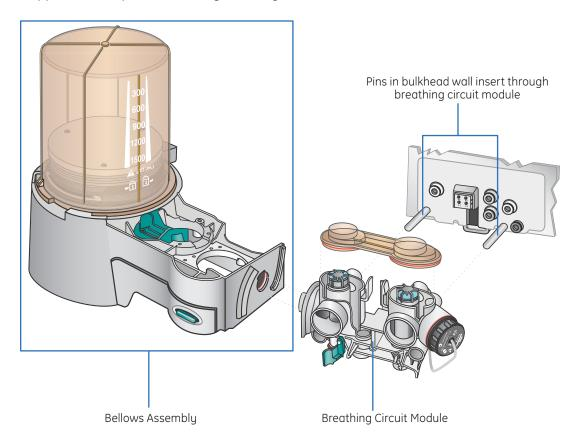
Figure 11.7 Replacing the Breathing Circuit
