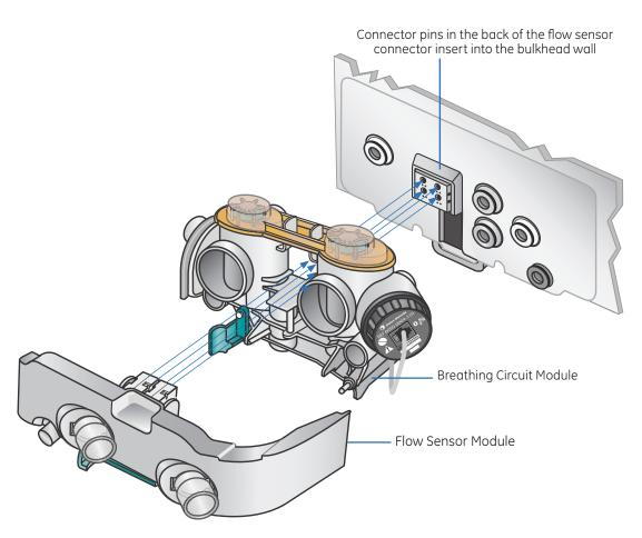
Figure 11.5 Replacing the Flow Sensors
