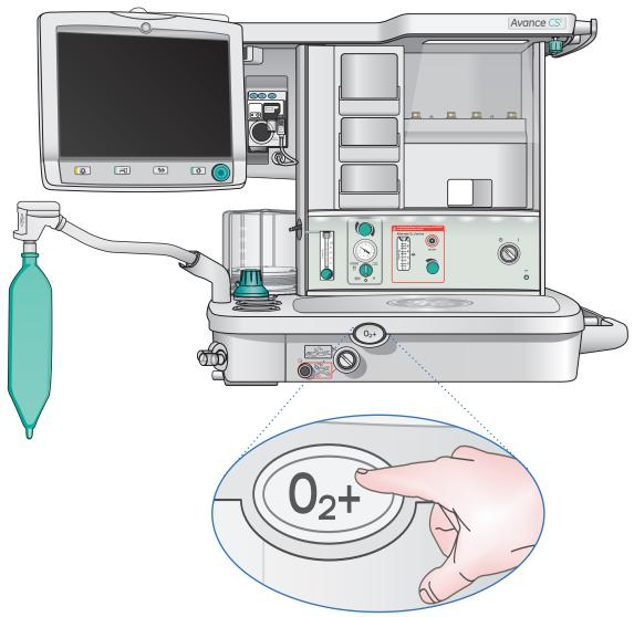
Figure 2.10 O<sub>2</sub> Flush Button
