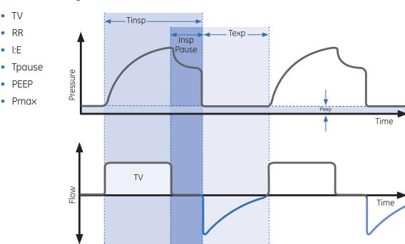
Figure 7.1 Example of Volume Control (VCV) Waveforms
