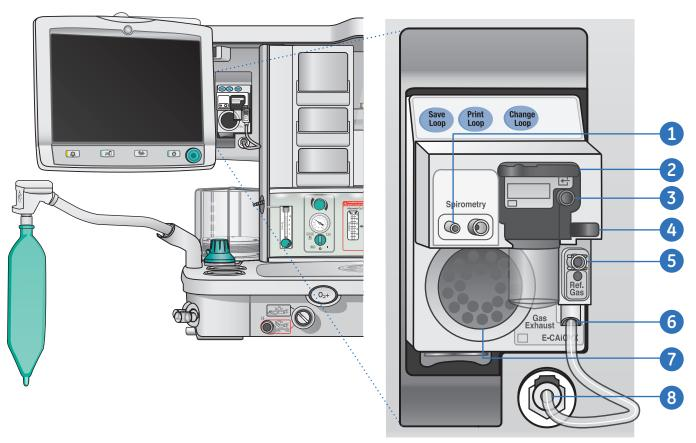
Figure 2.8 Compact Airway Module
