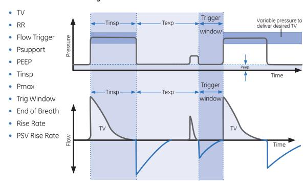
Figure 7.6 Example of SIMV-PCV-VG Waveforms
