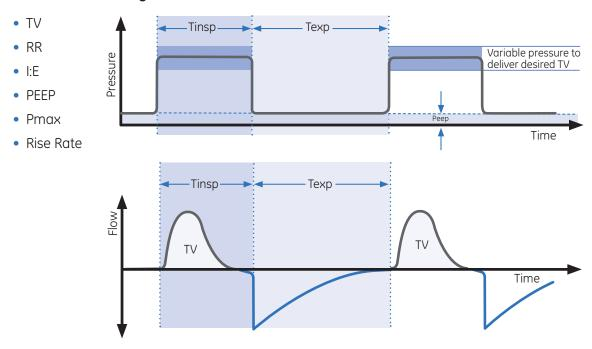
Figure 7.3 Example of PCV-VG Waveforms
